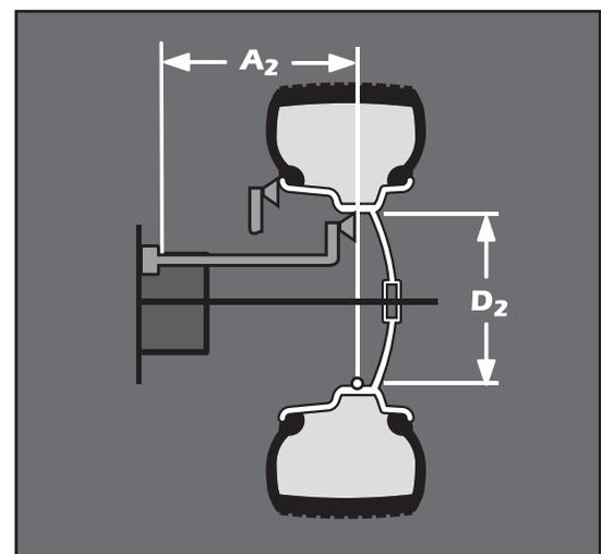
Figure 11 - T2 Tape (Hidden Tape-A-Weight®) Data Entry Diagram
