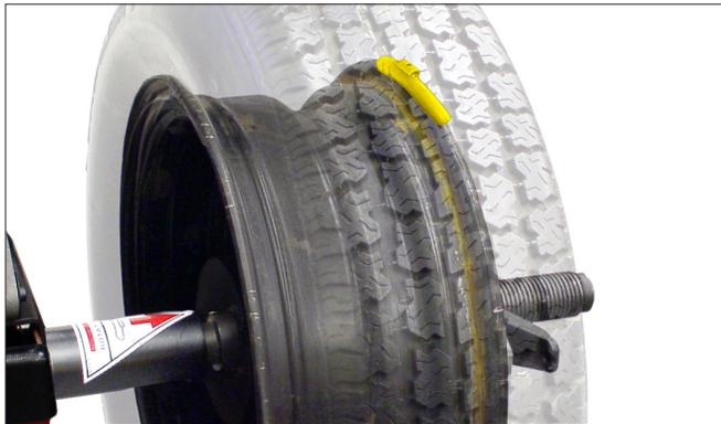
Figure 24 - Calibration Weight On Outboard Flange At Top-Dead-Center
