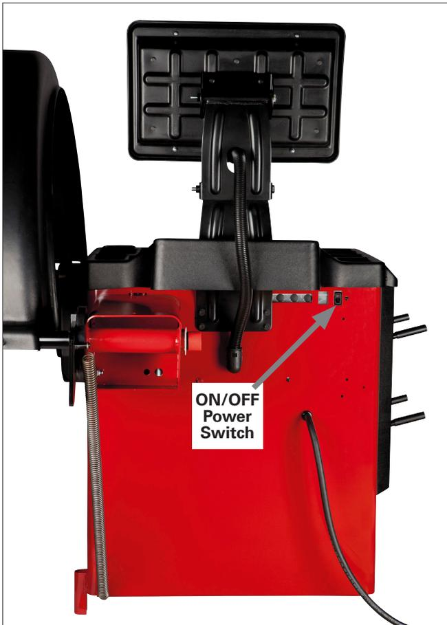
Figure 5 - On/Off Switch
