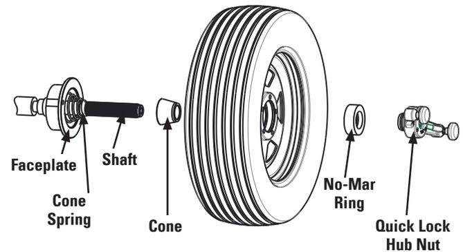
Figure 15 - Alternate Mounting
