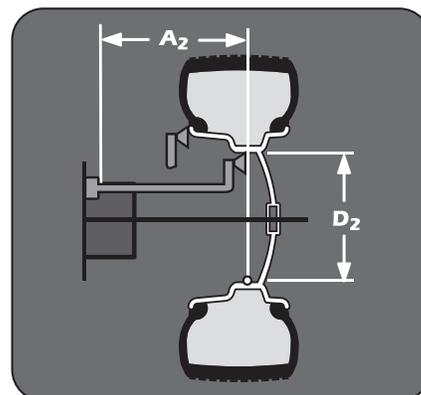
Figure 18 - A2 and D2 Tire Dimensions
