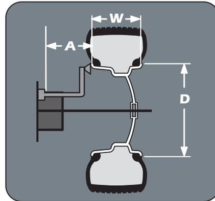
Figure 17 - W, D, and A Tire Dimensions
