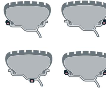
Figure 21 - Static Balance Weight Locations
