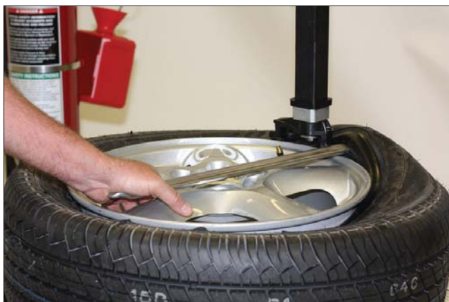
Figure 40 - Rotate Lifting Tool Down for Demount
