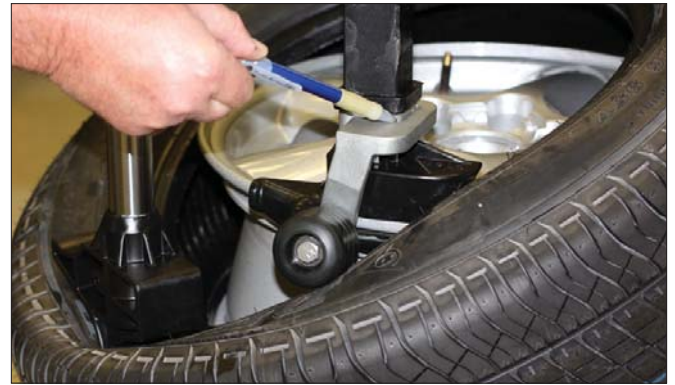
Figure 22 - Duckhead Roller Properly Mounted On Bracket
