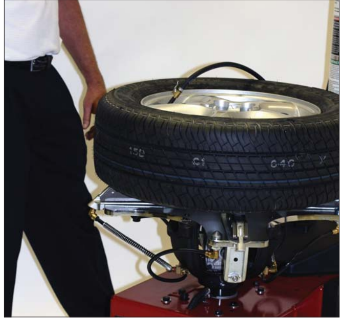
Figure 26 - Stand Back during Bead Seat
