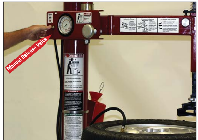
Figure 27 - Location of Manual Release Valve
