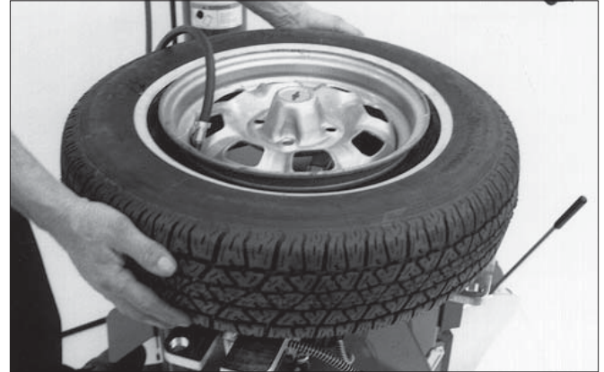
Figure 25 - Lift Tire Upwards for Bead Sealing
