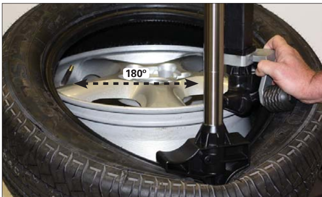
Figure 21 - Position Valve Stem 180° Ahead of Mount Tool
