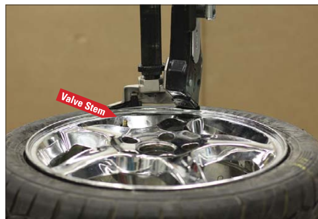
Figure 50 - Position Valve Stem Behind Leverless Demount Tool
