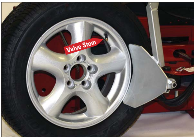
Figure 29 - Position Tire for Bead Loosening
