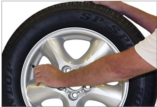
Figure 1 - Remove Valve Core to Deflate Tire
