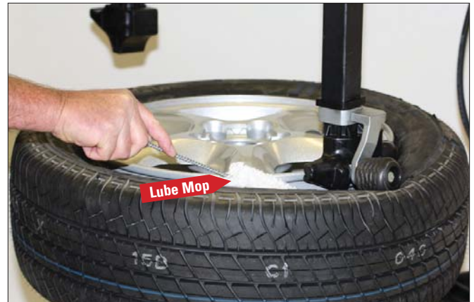
Figure 35 - Lubricate Upper Bead
