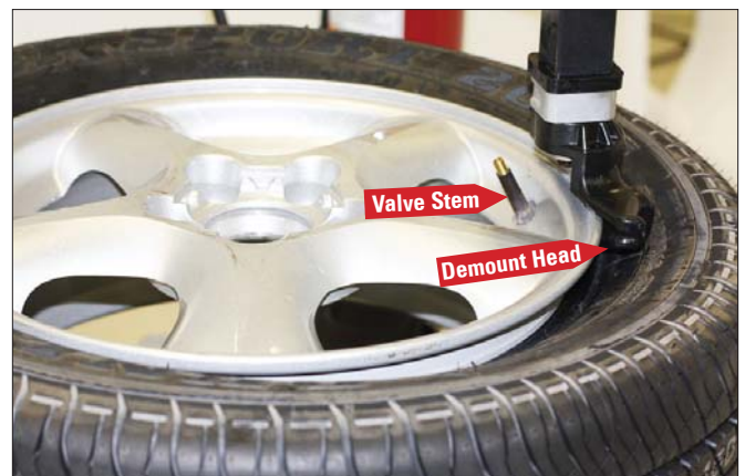
Figure 36 - Position Valve Stem Under Demount Tool
