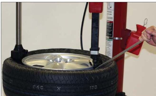
Figure 38 - Helper Foot Pushing Bead Into Drop Center
