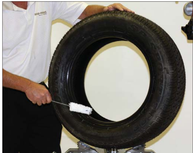
Figure 18 - Lubricate Tire Beads Liberally
