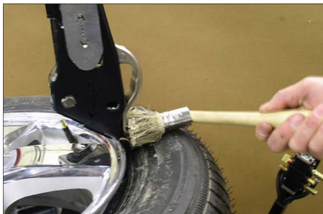
Figure 49 - Apply lubricant to Bead Lifter Tool Hook
