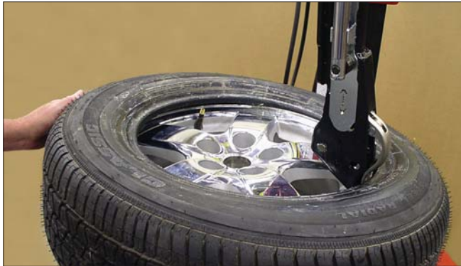
Figure 52 - Demount Upper Tire Bead
