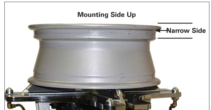
Figure 6 - Place Tire/Wheel Assembly on Table top
