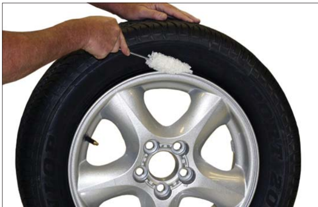
Figure 5 - Apply Rubber Lubricant to Tire Beads
