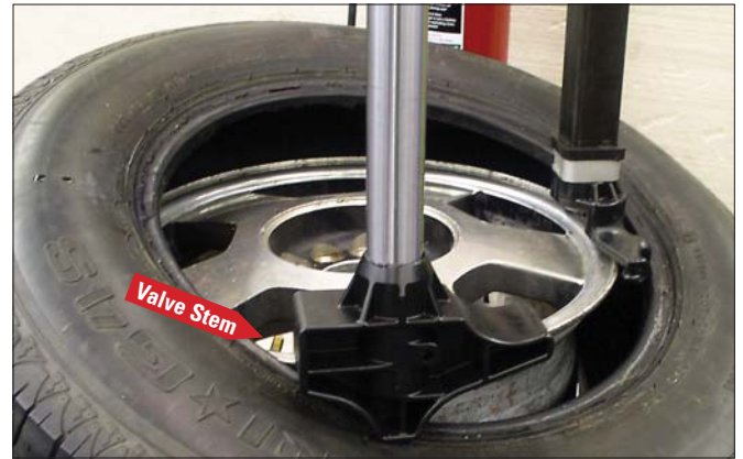
Fig 45 - Use Robo Arm To Hold Tire In Rim Drop Center
