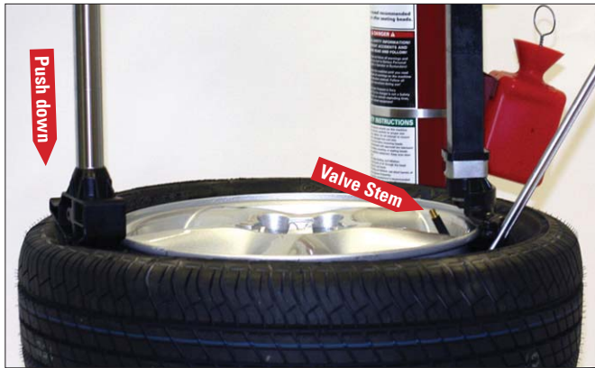
Figure 12 - Insert Bead Lifting Tool
