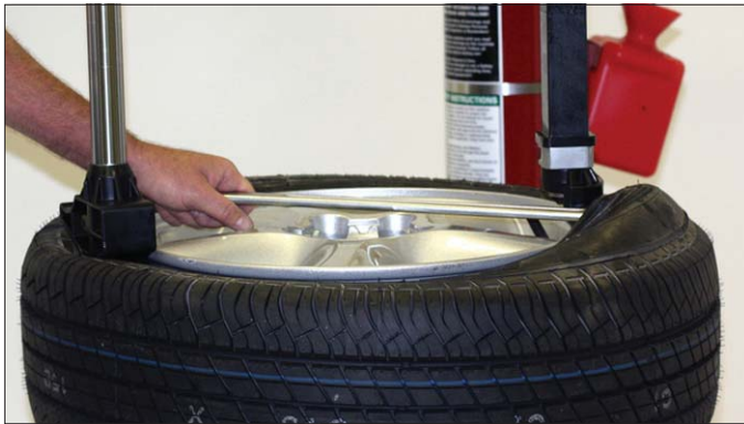
Figure 13 - Lift Bead Over Demount Tool
