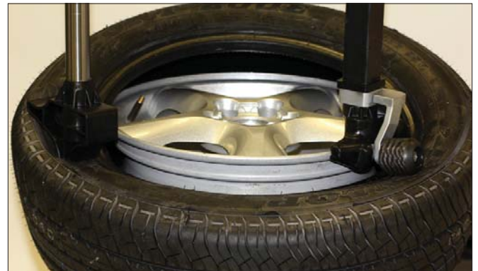
Figure 24 - Mounting Top Bead
