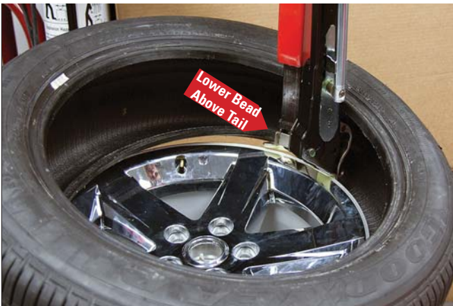
Figure 58 - Position Tire Against Bead Lifter Tool
